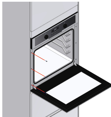
Screw the oven to the MFC side using the screws supplied by the Oven manufacturer
